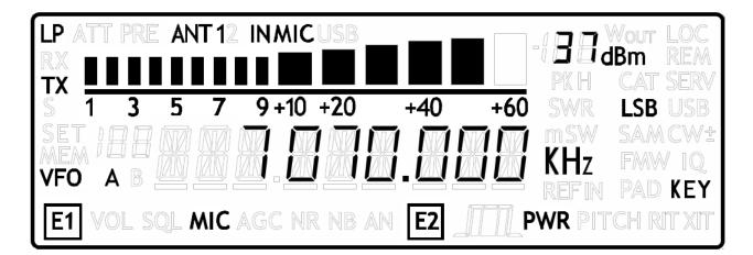
Before transmitting, always check the antenna conditions, so as to avoid problems to the PA; this must be done on a free frequency to avoid disturbing any running QSOs.
