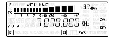
In this mode a tone at the transmission frequency is generated. Use E2 to modify the transmission power.
