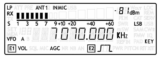
After some secs the device is in reception mode with VFO A enabled.
