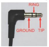
RING: do not connect (reserved for future use) TIP: PTT output (NPN Open Collector transistor, max.: 20V/200 mA)
